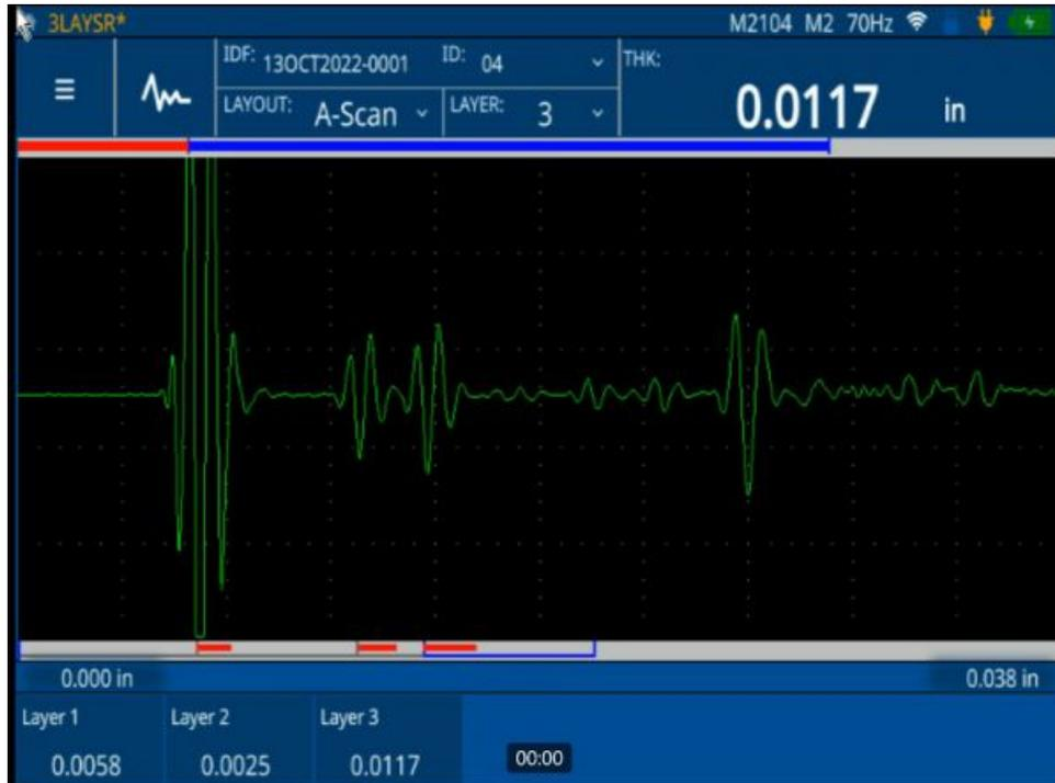
50 MHz measurement of a three-layer plastic container performed on the 72DL PLUS ultrasonic thickness gauge
